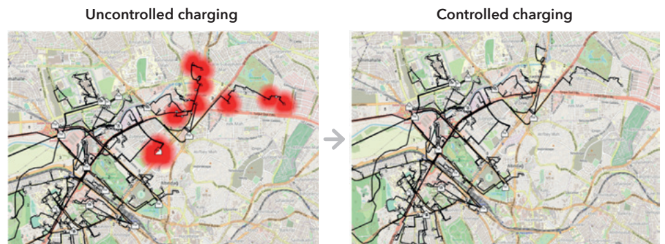
Figure 70. The impact of the e-mobility load on a portion of the distribution system in the Akköprü region: Smart (controlled) charging vs uncontrolled charging
