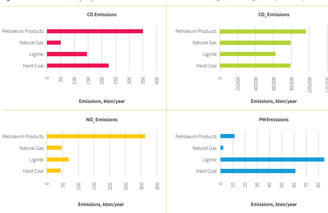
Figure 29: Emissions of CO, CO 2 , NO x , and PM based on the combustion of hard coal, lignite, natural gas, and petroleum products
