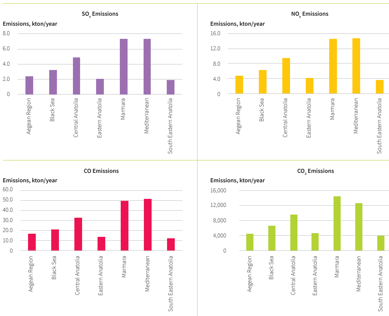
Figure 18: Regional distribution of some major pollutants and CO 2 emissions from the cement industry
