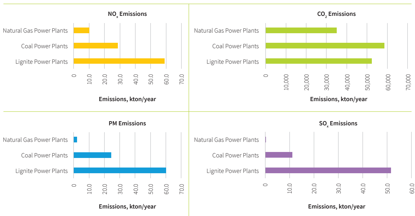
Figure 13: Distribution of major air pollutants and CO 2 emissions based on power plant type
